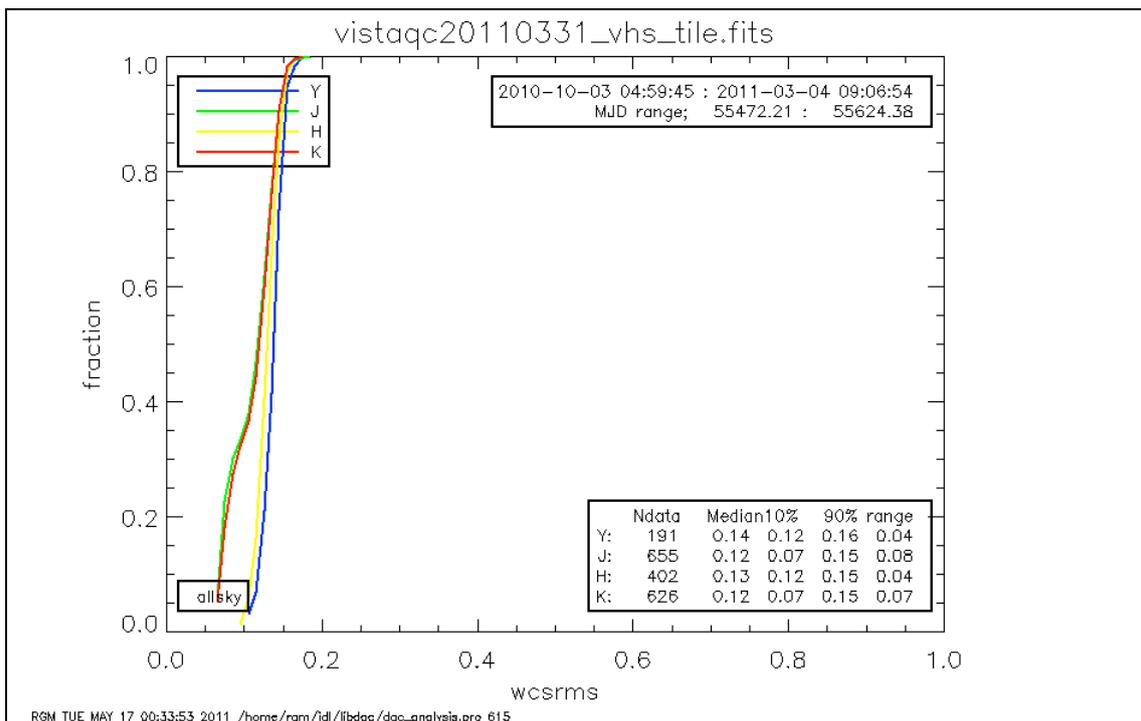
**Figure 8:** Distribution of the World Coordinate System (WCS) rms astrometric errors for tiles. The J and K bands have a tail to smaller values compared to Y and H due to larger fraction of fields at low galactic latitude and hence more WCS 2MASS astrometric calibration stars.
